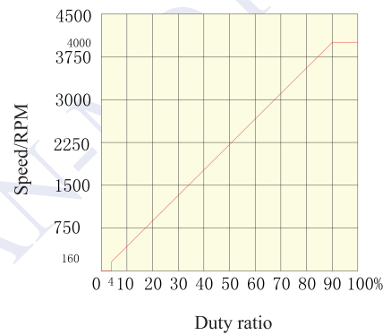
Relational graph between duty ratio and the motor speed (closed loop no load)
