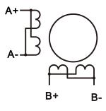
8lines stepper motor, in series (High torque output)
