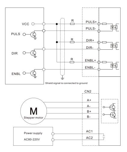
Step pulse signal is PUL, direction signal is DIR, offline signal is ENA. If the power supply is 5V, it can be directly connected. If the external system uses a PLC or other control voltage exceeds 5V, it needs to be outside Add a current limiting resistor.
